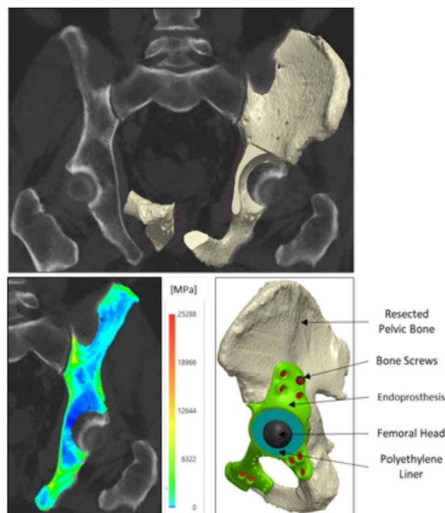
Fig. 1: Finite element model generation: 3D model of resected pelvic bone on a CT scan (top). The distribution of the material properties of the bone derived from the CT scan (left bottom). An implanted massive custom-made pelvic endoprosthesis (right bottom).
